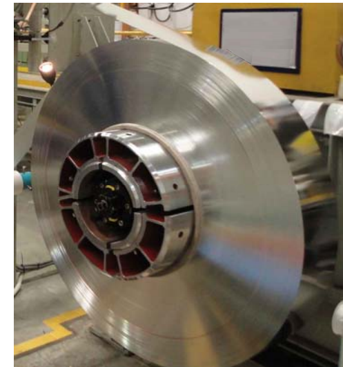
Copper rolled product being tin plated
