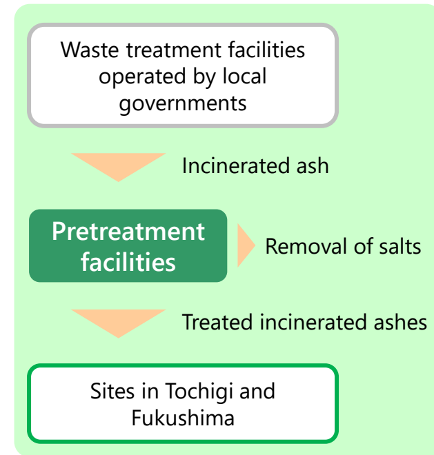
Positioning of pretreatment facilities in the melting/recycling waste business
