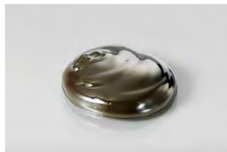
Silver nano paste for use as an alternative to solder
