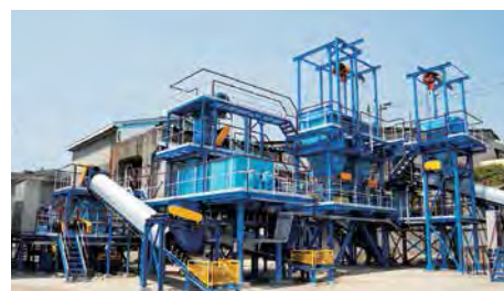
Eco-System Hanaoka Co., Ltd.'s soil remediation facilities, for which a unique remediation method was adopted
